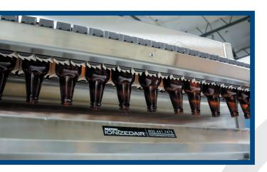
The process of aligning the system to the needs of a brewery facility required some tweaks along the way. For instance, the initial location of the system near the filler resulted in syrup gumming up the works. Relocating the blower to the opposite side of the filler resolved this initial issue.
